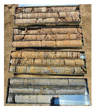
Lindfield Project drill core (hole LIND014) showing the oxidised core intersection from 5.8m depth which contains both Vanadium and Alumina.
